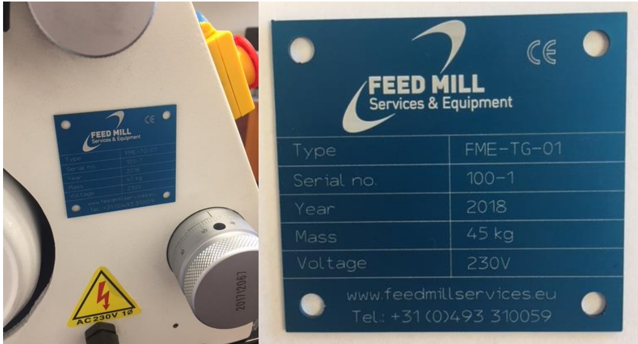
Figure 2.8.1 Example of a type plate
